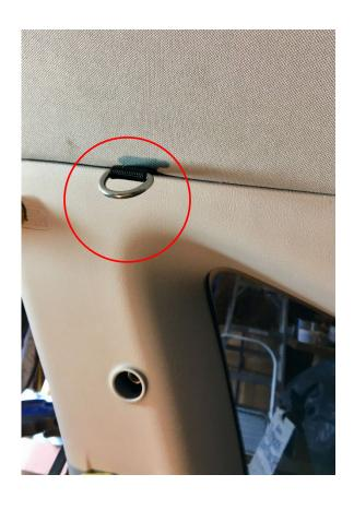
**Step 9**Install the upper seat belt bolts with the C1015 brackets installed as shown on the driver's side
