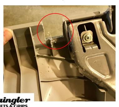
**Step 8**Reassemble trim panels with strap and D ring over top of trim
