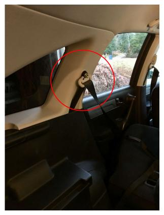
**Step 2**Unbolt the bolt and drop the seat belt assembly out of the way
