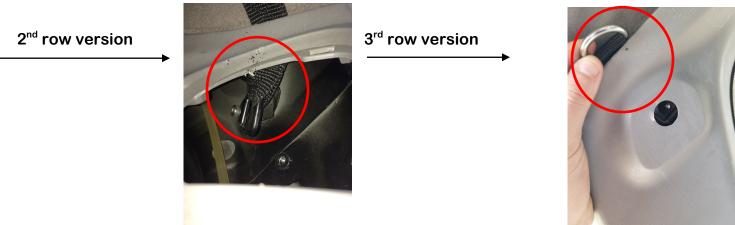
Reinstall with the D ring tether protruding over the top of the D pillar trim and reassemble.  $3^{\rm rd}$  row version shown here.
