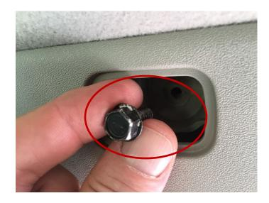
Fit the included Raingler C100XL hardware mount over the black 10mm bolt.
