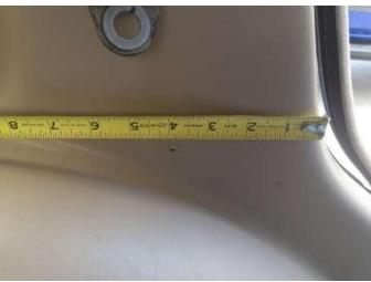
The hole will have to be enlarge incrementally to 1/2" through the outer plastic trim and the inner structure. Again, be careful to check clearance and go slowly as to not damage wiring, washer hose or outer sheet metal damage.
