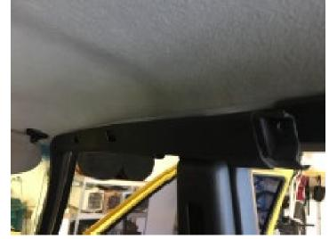
Locate the best area to install the C100X hardware. You can install it right at the back of the front door, or at the front of the rear door. Either location works. See photos. Mark your hole with a Sharpie pen before drilling.
