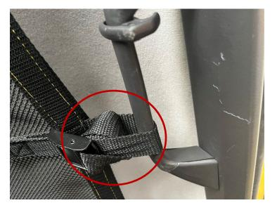
Lastly, run the front straps through the front hardware you installed.
