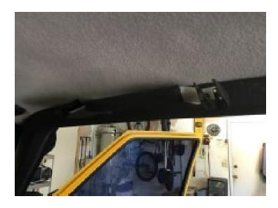
Also remove the screw in the panel toward the back seat as shown. Pop the pillar out and back to allow room to work.
