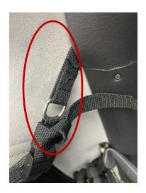
Next, run the straps through the hardware you installed at the rear seat belt. Do this on both sides.
