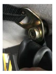
Alternate installation: turn the mount toward front of vehicle, for easier access. This alternate installation also is useful if you are using the same mount for a ceiling net installation.
