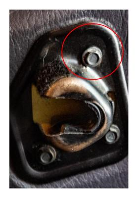
**Step 4**Add the square ring to the REAR bolt (closest to cargo area). Tighten bolts
