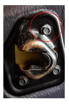
**Step 4**Add the square ring to the REAR bolt (closest to cargo area). Tighten bolts down.
