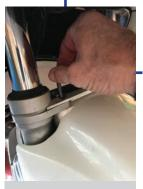
Fig. 10 Install two new bolts into the open holes, then remove the mounting studs and install the remaining new bolts. This requires a 7/16 or 11-mm-thin wall socket.
