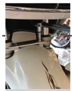
**Fig. 11** Torque the bolts to 12 feet/pounds.
