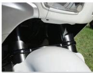
PROS: Sturdy reinforcement of the front forks, giving you firmer control and feedback in turns, cornering and over various road surfaces. Minimizes any wobbling or vibrations, as well as flexing of the fork tubes, which can lead to bending or premature leaking around the seals.
