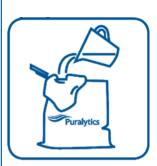
Remove the cap and insert the pre-filter into the Solar-Bag, fold elastic edge over the SolarBag opening to hold in place. Pour the source water through the pre-filter until the SolarBag is full. Remove the prefilter and replace the cap.
