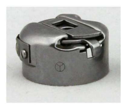
The spring for the towa bobbin case is round with 2 little arms bent out slightly from each side like this:
