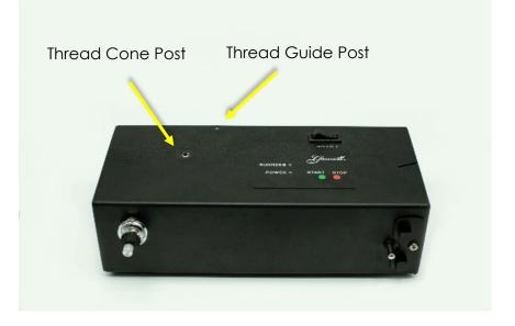
You will need to unwrap the power cord and plug into the outlet on the left side of the bobbin winder. Once the power cord is plugged into the bobbin winder and an electrical outlet, you can use the main power switch just above the power cord to turn on the bobbin winder.
