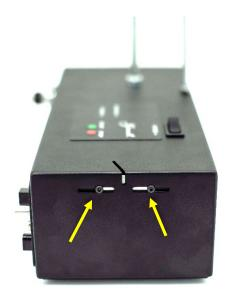
When the thread cutter becomes dull, the blade can be adjusted to provide a fresh, sharp cutting surface. Using a 2mm allen wrench, loosen the two screws holding the cutting blade. Do NOT completely remove the screws! Slide the blade either to the left or the right. Re-tighten the screws to hold the blade firmly in place.
