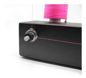
To adjust the tension of the Professional Bobbin Winder, turn the black knob clockwise to increase tension or counter-clockwise to decrease tension. You can use the silver knob to adjust the centering of the thread on the bobbin.
