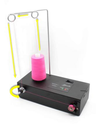
Now, it's time to wind bobbins! First, slide the thread through one of the holes in an empty bobbin from the inside toward the outside. Next, while holding the thread, place the empty bobbin on the motor spindle and push all the way on.
