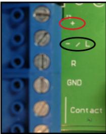
Balanced Audio Input: (Most often, but not always characteristic of paging systems.) Connect signal wires to + and - at the input. Connect the shield to GND at the audio source.
