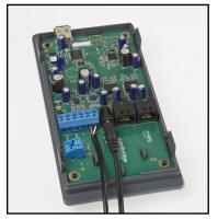
The controller comes standard with a 24 V wall plug power supply. This supply features a wall plug and a fixed barrel connector.
