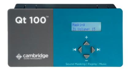
The Qt® 100 control module is a sound masking generator, controller and amplifier, with one auxiliary audio input to allow for distribution of audio from a paging controller or (background) music player. The Qt 100 control module is a compact one-zone controller suitable for installations of up to 12,000 square feet (1,115 m²). The masking level can be adjusted from the unit's front panel. Auxiliary audio level is set via the front panel.
