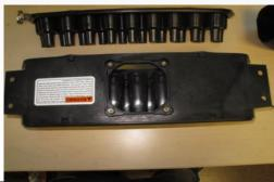
**6.** Rinse off the particle separator, plenum, and back plate with low pressure water at an angle to remove any debris. Do not spray water directly at the tubes as this may dislodge the tubes from the housing.
