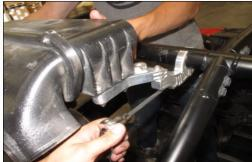
$5.\,$  Loosen the screw for the passenger side factory frog skin side cover. Lift up and pull towards the front of the vehicle to remove the frog skin side cover.
