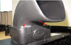
5. Remove the fan exhaust and fan. Note where the fan harness is located and how the fan is sitting on the housing. The fan guard is installed on the exhaust side of the fan. Do not remove the fan guard. Removal of the fan guard will not increase the performance of the particle separator. The fan must be reinstalled the same way it was disassembled.
