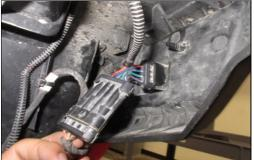
19. Locate Connector B and run the wire along the back of the fender well to the hole that leads to the battery compartment. Feed the connector through to the other side. Use Cable Ties (S) effectively to secure the harness. Route the harness so that the wires will not get damaged or pinched while the UTV is operating. Keep it away from any exhaust components or moving parts.
