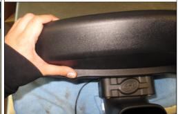
16. Reinstall the five screws and washers that were taken out. Do not over tighten and make sure the screws are on finger tight (20 in-lbs). The cleaning is complete.
