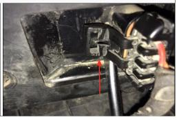
18. Connect the male factory connector into the Connector A female connector. Then install the Connector A male connector into the tail light assembly. Use Cable Ties (S) effectively to secure the harness. Route the harness so that the wires will not get damaged or pinched while the UTV is operating. Keep it away from any exhaust components or moving parts.
