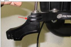
3. Insert the Tube Clamp Screw Side (N) into both the left and right Clamp Adapter (M) through the ridges. Push in the Screw (R) through the backside of the clamp adapter and install the Tube Clamp Nut Side (O) with a 6mm hex key. Only turn the screw a couple turns to leave enough room for the clamps to go around the roll bar.
