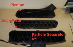
3. Once the back plate is removed, blow compressed air into the particle separator to remove any noticeable debris. Using water is not recommended to clean the particle separator with the fan installed.
