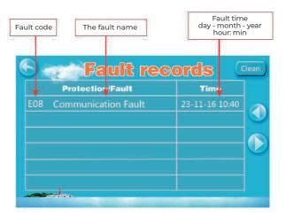
If no failure, main interface displays static "🛕" When fault occurs, the fault icon will flash between the " $\triangle$  " " $\triangle$  ", the failure interface will record time, code, name of the fault. After troubleshooting, if you do not check the failure record, the main interface will display static " 1 "; if you check the failure record, the main interface will displays static " $\triangle$ ";
