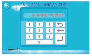
Click the value to set time directly, the click confirm button to save the Settings. For example: setup time: the 30-11-2016 16:00:00, input 30 11 16 16 00 00, the time change then click confirm button.
