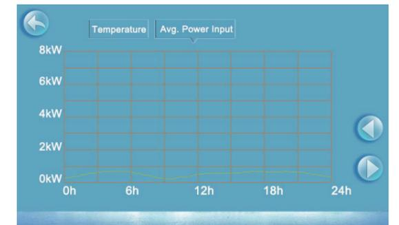
Temperature curve automatically updates every one hour, and the curve record can be stored for 60 days;
