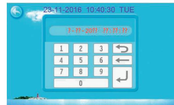
Click the value to set time directly, the click confirm button to save the Settings. For example: setup time: the 30-11-2016 16:00:00, input 30 11 16 00 00, the time change then click confirm button.
