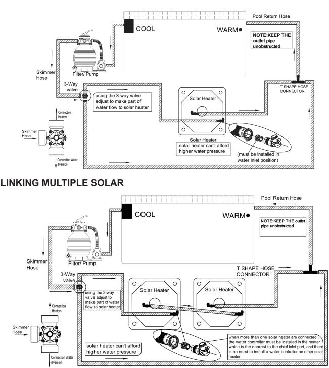
**NOTE:** The connections here show the water flowing into the Solar Heater through the center connector and out through the side hose connector. This diagram is for reference only as the flow may be reversed if you choose (i.e. the water flow coming in through the side hose connector and out through the center hose connector). The **WATER CONTROLLER** must put into the water inlet position.
