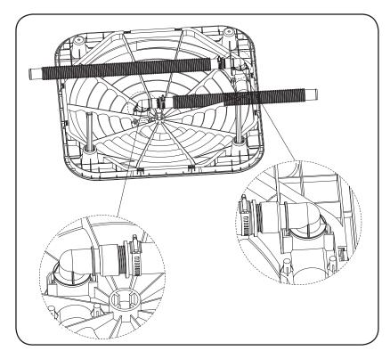
NOTE: The short hose is only used to connect multiple solar heaters together.
