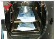
Follow your Autoclave instruction manual for the best Pouches should never touch the Autoclave or be position for pouch placement.
