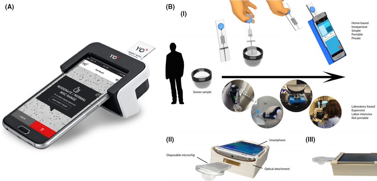
Figure 5 Smartphone-based devices. (a) YO Sperm Test attached to smartphone with slide inserted. Once the test is complete the application will report the concentration of motile spermatozoa and indicate if it is within the normal range, as well as show the user a recorded video of their spermatozoa. (b) Device by Kanakasabapathy et al. (i) A comparison of steps of the smartphone-based device and traditional methods. Semen sample is loaded onto smartphone-based device using bulb and then the microchip is separated from the loading end and placed in the optical attachment. Sample loaded into counting chamber and microscope and then evaluated manually or with a CASA system. (ii) Actual device with smartphone, microchip, and attachment. (iii) Side view of device. Reprinted with permission from Medical Electronic Systems (Information Obtained from Weblink) and Kanakasabapathy et al. (2017b).
