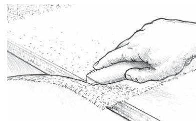
Figure 26 Trim excess cloth after the epoxy gels.
