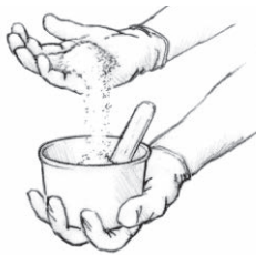
Figure 5 Stir in small handfuls of filler until the desired consistency is reached.
