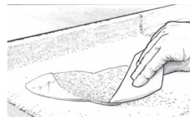
Figure 24 Spread the epoxy over the cloth surface with a plastic spreader.
