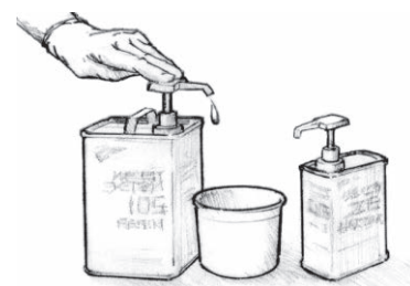
Figure 2 Dispense the proper proportions of resin and hardener.
