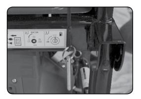
Loop the pin strap around the generator frame next to the handles and then pass the pin through the strap to secure it to the frame.
