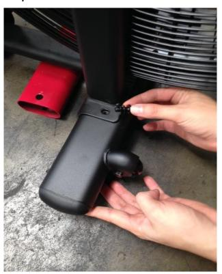
**Step 9:** Using the provided 6mm Allen wrench, tighten the two #58 Screws, two #34 Lock washers, and two #35 Flat washers to secure the front stabilizer bar.
