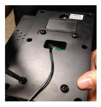
**Step 20:** When installing the Computer Console, tuck the excess length of Speed Sensor cable into the Computer Mast.
