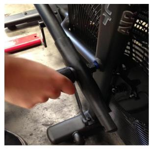
**Step 25:** Using the provided multi-tool tighten the 22mm nut between the handle bar and the frame. **NOTE:** Make sure to tighten this nut tightly so there is no movement and there are no threads exposed.
