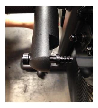
**Step 27:** Once the #37 Pivot Pin and #84 washer onto the handlebar install the linkage arm.
