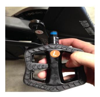
Step 34: Install the #16 Left pedal onto Left crank arm by threading it loosely COUNTER-CLOCKWISE and then use the Multi-tool to tighten it the rest of the way. Make sure it is installed tightly. NOTE: Only the left side is reverse threaded.
