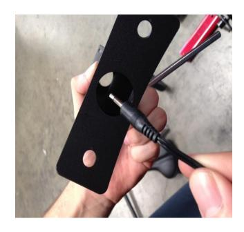
**Step 14:** Pull the Speed Sensor cable so there is no slack in the cable.
