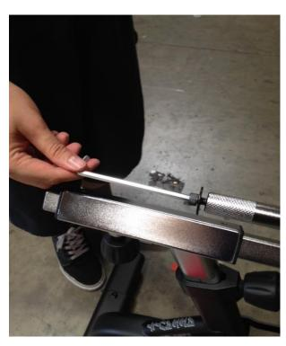
**Step 30:** Using the provided 6mm wrench, remove the 6mm Allen screw and washer from the Seat post Assembly.
