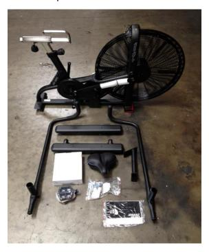
Step 6: Using the provided multi tool remove the nuts securing the red transport tube. Note: After assembly this red tube can be discarded and will not be used along with the nuts and bolts that held it in place.
