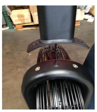
**Step 15:** When installing the Computer Mast make sure the Speed Sensor Cable does not get pinched between the frame and the mast.
