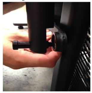
**Step 28:** Once the #37 Pivot Pin is inserted into the linkage arm install the #84 washer and then the #85 locknut.
