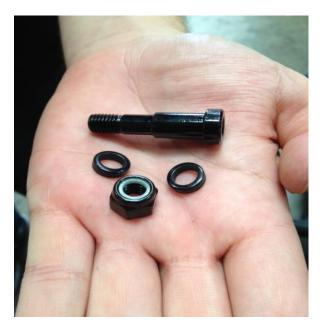
**Step 26:** Install the #37 Pivot Pin and #84 washer onto the handlebar.
