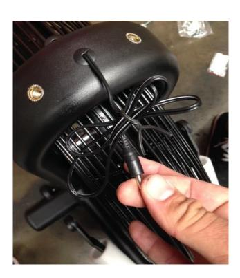
**Step 13:** Route the Speed Sensor cable through the console mast.
