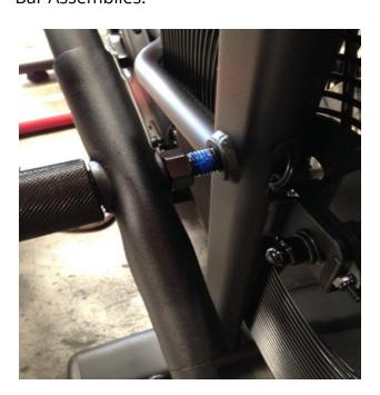
**Step 24:** Install the Handle Bar Assemblies by rotating the peg Clockwise. **NOTE:** Make sure they are being threaded on straight and are not being cross-threaded.
