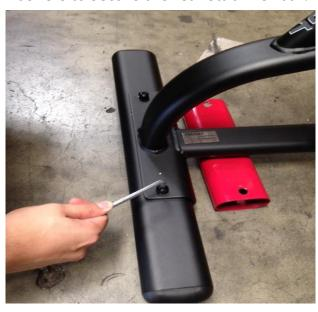
**Step 12:** Locate the speed sensor wire and remove the twist tie.
