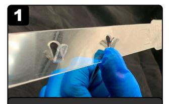
Bend the four tabs out to a 45° using a small screwdriver.
