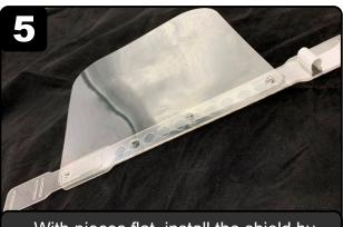
With pieces flat, install the shield by starting at one side and hooking the holes on the tabs.
