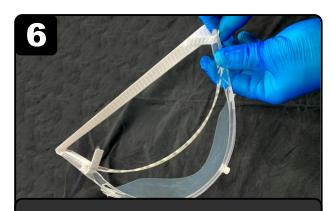
Bend the headband to lock the shield in place and install the elastic on other side.
