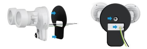
3. Before securing the cover of your junction box, thread the wires through the slot on the bottom of the plate to access them during installation.
