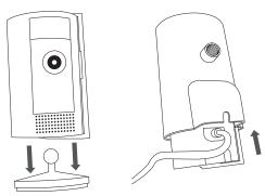
3. Close and secure the screws at the bottom of the case. Make sure the cable sits in the groove at the back.
