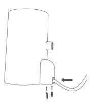
4. If you install the camera outdoors, mount the wall mount with the screws and anchor provided. Ensure to route the cable lower than the case to prevent water from getting into the case.
