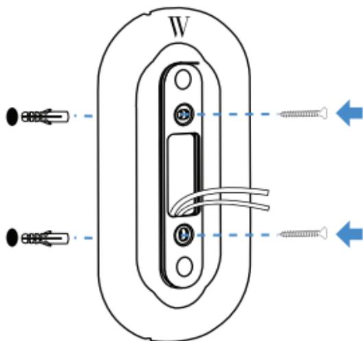
5. Connect the wires to the doorbell. Then, attach the doorbell to the wall plate as shown.
