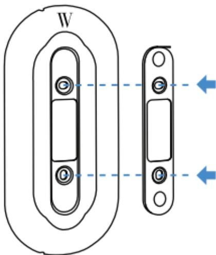
4. Feed the wires through the cutout as shown below. Mount the wall plate along with the backplate to the wall using the screws and wall anchors provided (the drill bit size is 1/8 in).
