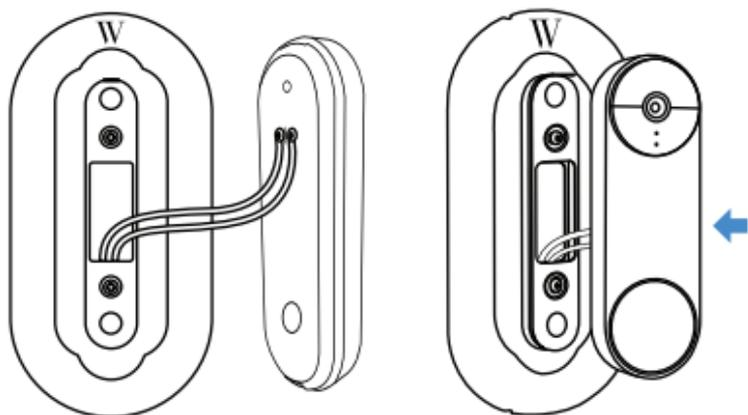
5. Secure the doorbell with the screw that came with your doorbell. Turn on the power and check the App to make sure the doorbell have been installed properly.
