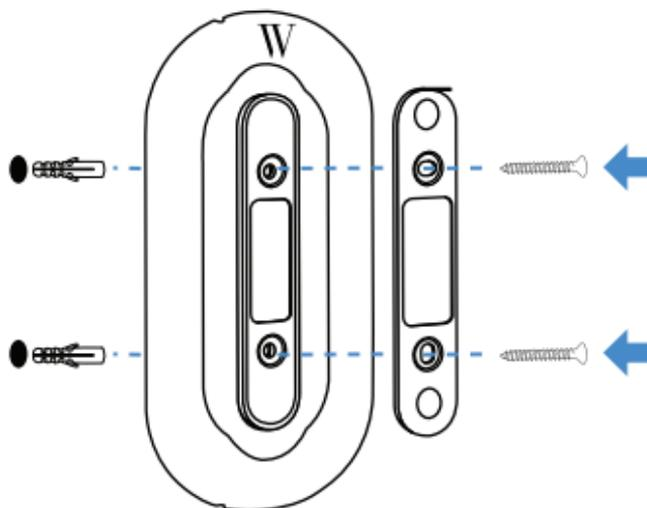
4. Connect the wires to the doorbell. Then, attach the doorbell to the wall plate as shown.
