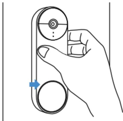
3. Align the doorbell backplate with the wall plate.
