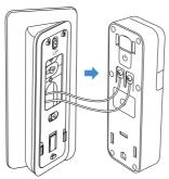
4. Turn on the doorbell. Hook the tabs at the back and press firmly until it clicks into place.
