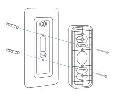
Screw the doorbell's backplate onto the angle mount using the original screws that come with the doorbell.
