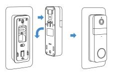
5. Check the view from the App, then secure the doorbell with a screw at the bottom.
