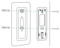
2. If you have a wired doorbell, connect the wires first before securing it to the wall plate.
