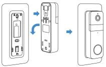
4. Check the view from the App, then secure the doorbell with a screw at the bottom.
