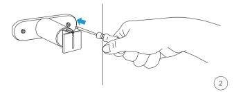
4. Slide the solar panel onto the mount attachment.
