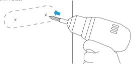
3. Insert wall anchors and screw mount to the wall.
