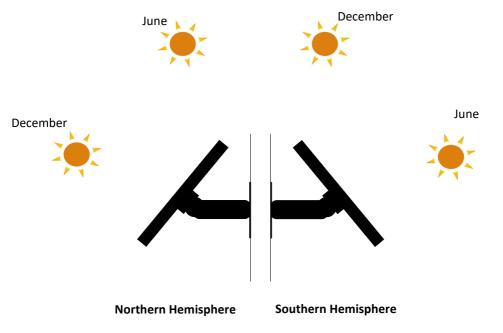
The amount of energy that the solar panel can produce is determined by sunlight exposure, weather conditions, etc. You have to consider where to place your solar panel according to geographic location. To maximize the power generated by your solar panel, please do the following:
