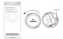
Once connected, tap on the "Done" icon on your mobile phone to enable connection to the sensor.
