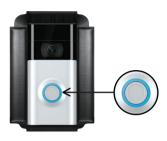
However, when the solar charger is charging the Doorbell 2nd Generation, this light flickering may NOT HAPPEN every time. At times when there is no light flickering, use your Ring App to check if the battery life has been extended.
