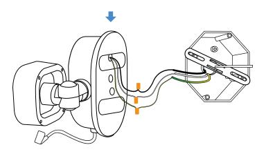
5. Mount the floodlight onto the crossbar and secure it with the screw cap provided.
