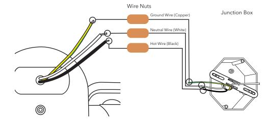
4. Make sure that the wire connections are secured. Carefully place the wires into the junction box.
