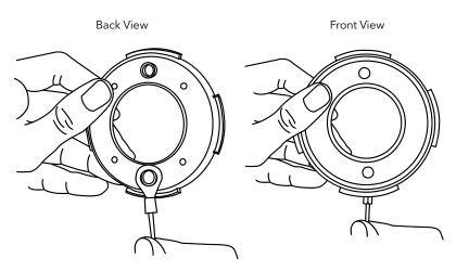
$2. \ \, \text{Screw in the wall plate tightly using the two short screws provided}.$
