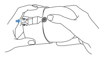
5. Make sure that the end of the security chain with the small hole goes in between the screw holes of the mount. Use the hexagon screwdriver to tighten the mount and lock the security chain.
