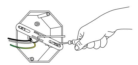
3. Ensure that the center screw hole and wire slot of the foam gasket are aligned with the screw hole and wire slot.
