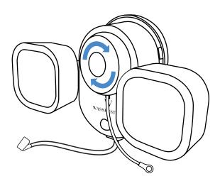
4. Slide in the anti-theft mount on the camera, make sure to align the speaker/cable opening at the bottom.
