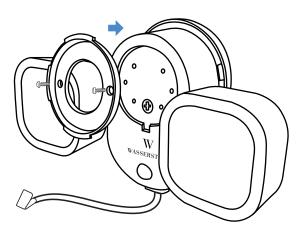
3. Attach the magnetic plate onto the wall plate and turn it clockwise to lock it in place
