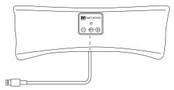
During the charging process, the control box indicator will be red, indicating that the device is charging.
