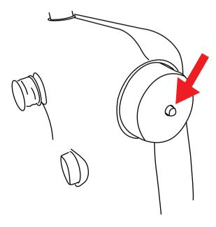
3. Place an empty metal bobbin on the raised Bobbin Holder and put the thread around the metal bobbin as below.
