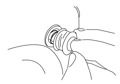
4. Pull the thread through the first thread guide ①.
