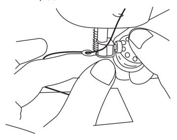
3. Place the new needle with the flat side facing in against the needle clamp (P). Push the needle up gently as far as it will go, and against the needle clamp (P). Tighten the needle clamp screw (O) while holding the needle (R) in place.
