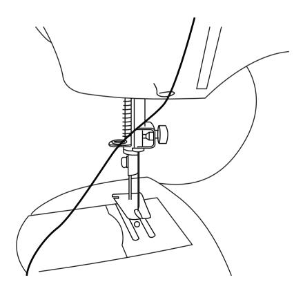
9. Pull the thread through the needle eye ② using the threader from the front toward the back of the machine. You can raise the needle (R) by turning the handwheel (K) clockwise.
