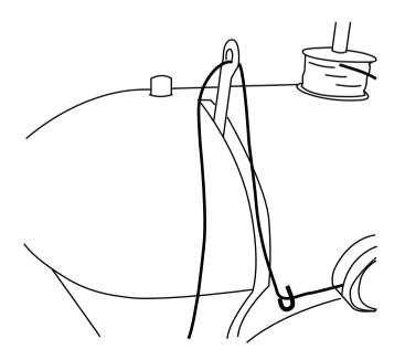
7. Pull the thread down to the thread guide ⑤.
