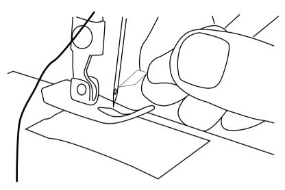
10. Pull approximately 9.84 inches of thread through the needle (R) and lay it on the deck under the presser foot (F).
