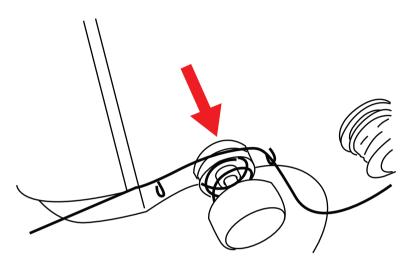
6. Pull the thread in the direction towards the front of the machine through the thread guide ③. After that pull the thread through the thread guide ④.
