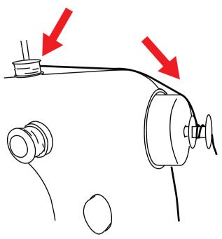
4. Once you have some thread on the metal bobbin, turn the Hand Wheel (K) clockwise to start transferring the thread. To automate this process, you can power the sewing machine and connect the foot pedal. Pressing on the foot pedal will automatically rotate the Hand Wheel (K) to thread faster.
