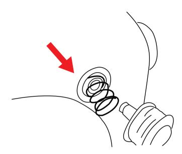
2. Attach the spring back and place your metal bobbin with thread on the Bobbin Spindle.
