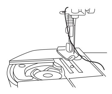
2. Turn the handwheel (K) clockwise. The needle will go down, picking up the bobbin thread. Continue to turn the handwheel until the needle (R) has descended fully and then returned to the highest raised point. Raise the presser foot (F) and bring the spool thread around to the front. Pull it gently up and you will see that it has caught the bobbin thread. Pull the two threads towards the rear (away from you) and lay them under the presser foot (F).
