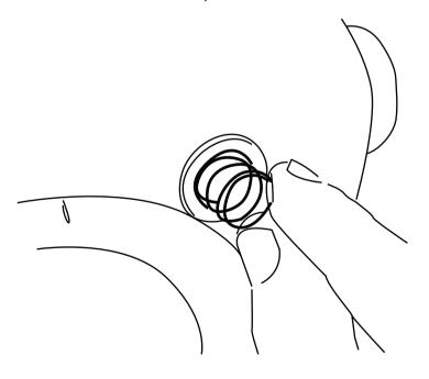
3. Place the metal bobbin together with the Bobbin Spindle back to the Bobbin Holder (V).
