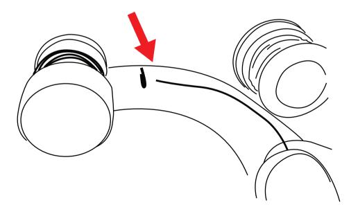
5. Pull the thread through the second thread guide ②. Here the thread goes over the tension screw (N) and must be positioned between the two washers.
