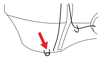
8. Pull the thread down through the thread guide 6.
