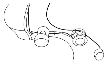
1. Pull out the metal bobbin from the Bobbin Holder (V) and be careful not to lose the spring.
