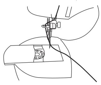
Note: It is important that the top and bottom threading is correct. Check carefully and practice before beginning to sew. Improper threading will damage the lockstitch.
