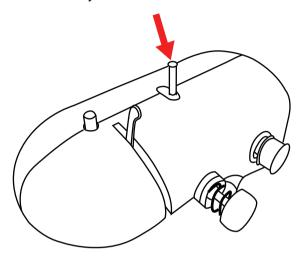
2. Press on the Bobbin Winder Spool (T) and turn it clockwise to release the Bobbin Holder.
