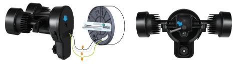
*Important:* Before mounting the floodlight, completely apply the EVA gasket around the perimeter of the cover plate where the back of the cover plate meets the mounting surface. This prevents water from seeping into the junction box.
