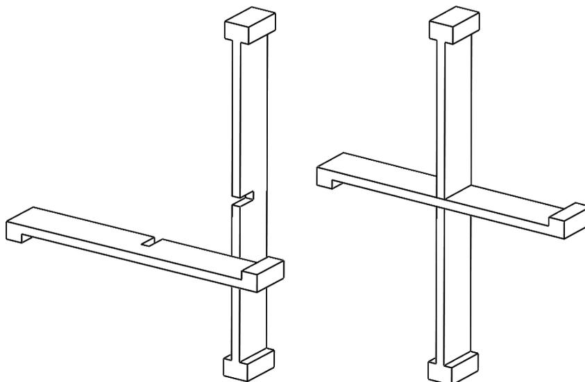
2. Locate the shortest internal support piece and place it on the assembly. Install the short screw through the hole in the short piece. It does not matter which other piece this part is screwed into.
