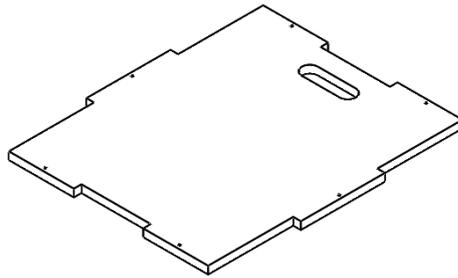
2. Locate one of the 20 inch panels with corresponding reference numbers. Install this panel into the slots of the 24 inch panel.
