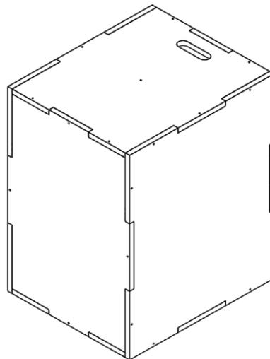
8. Insert all of the screws around the edges to secure the 24 inch panel.
