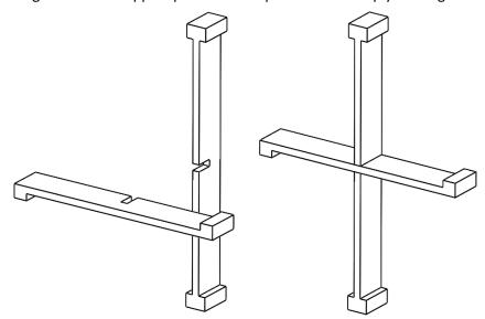
2. Locate the shortest internal support piece and place it on the assembly. Install the short screw through the hole in the short piece. It does not matter which other piece this part is screwed into.
