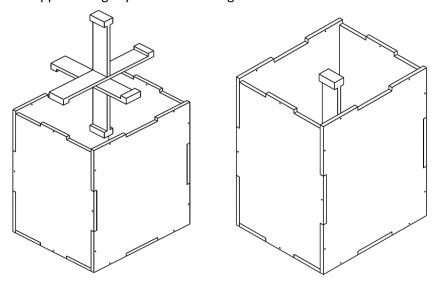
7. Locate the other 24 inch panel WITH the central screw hole. Slot this panel into the top of the assembly. Ensure a snug fit with gentle taps.
