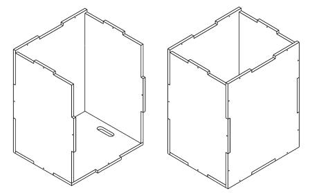
**TIPS & TRICKS:** It helps to leave the panels slightly loose to assist assembly. Once they are all together, a gentle tap will snug the panels together. The assembly should hold itself together before any screws are inserted.
