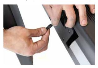
4. Align the right post assembly with the bolts on the running platform, Ensure the sensor wire is hidden within the cavity and not caught between the right post assembly and running platform. Affix the bolts provided and tension.
