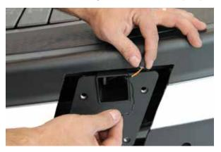
2. Free the sensor wire from the right Post assembly taking all precautions to ensure the wire is not damaged in any way.
