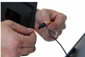
**10.** Push the excess sensor wire back into the frame (so that it is free and cannot be damaged in any way)
