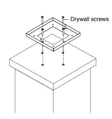
4. Attach the drywall screws through the holes of the metal plate and secure the drywall screws to the anchors.
