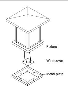
2. Remove the wire cover and metal plate from fixture, expose the wires.
