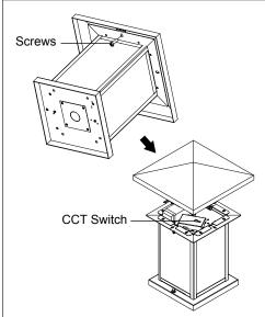
Remove the screws, Adjust CCT switch near the driver of fixture accordingly to the desired color temperature. Then tighten the screws.
