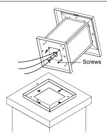
Connect the cover to the fixture with four screws, make sure the wires through the circle hole of the cover. Make all wire connections to appropriate wire. Secure with wire nuts(provided). Then tuck all connections neatly into junction box.
