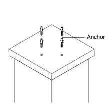
3. For mounting the metal plate to the wall, mark four spots. Drill four holes on the target. Insert four anchors through the holes of the wall.
