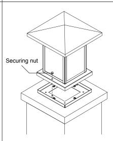
6. Use two securing nuts with rubber washers to tighten up the bracket to the wall.
