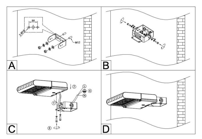
The mounting method of the straight arm is added to a wall mounted fixing plate, and the fixing plate is mounted on the wall, and the fixing plate is fixed by a nut.
