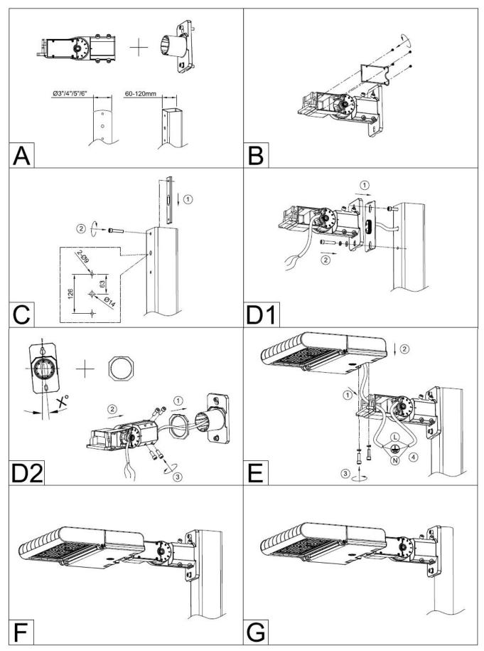
(2) Mounting with Slip fitter and Wall-mounted adapter:
