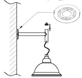
**Fig.8** Connect and fix the fittings with screws as shown
