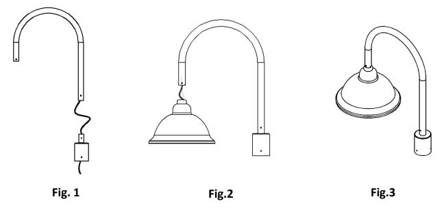
Connect and fix the fittings with screws as shown
