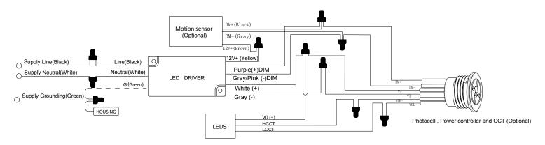
With sensor and Photocell/Watt/CCT controller
