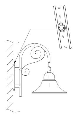
**Fig.12** Connect and fix the fittings with screws as shown
