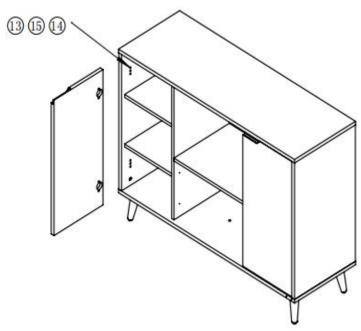
5. Each hinge (3) are installed in the corresponding position of the door panel with (15).
