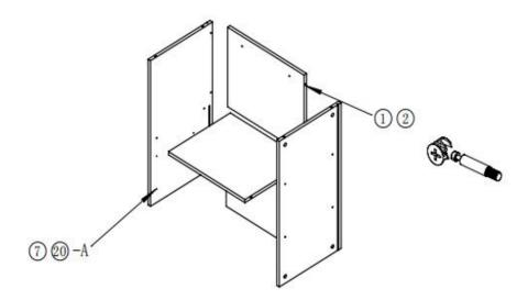
2. Install sliding rail ②-A on the inside of the 6 and 7 using ⑦. The 6 is connected with the 9 and 19 using ① and ②. The 7 is connected with the 9 and 19 using ① and ②. Insert the 20
