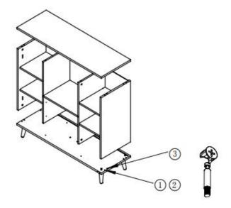
4. The 2 adopts ①, ② and ③ to connect the 4 and 8, At the same time, ① and 2 are used to connect the 6 and 7. Then Insert the 12 and 20. The 3 adopts ①,② and ③ to connect the 4 and 8. At the same time, ① and ② are used to connect the 6 and 7.
