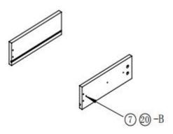
6. Install sliding rail ②-B on the outside of the 14 and 15 using ⑦.
