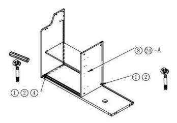
1. Install drawer slide 4-A in the corresponding position of the 12 using (8).
