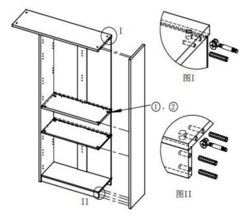
9. The 21 is connected to the cabinet with (1), (2) and (10). Note: The cabinet can be put down to fix the buckle wheel under the 3.
