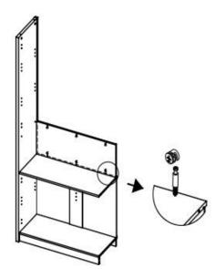
5. The 6 is connected with the 7 by (1) and (2).
