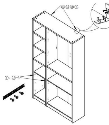
13、a. Install three pairs of sliding rail (1)-A on the inner side of the 1 and 20 by using (6).
