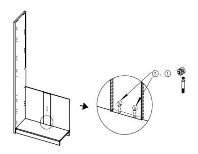
3. The 11 is fixed on the 3 with (1) and (2), and then inserted the 14.
