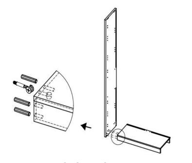
2, The 1 adopts the (1), (2) and (0) to connect the 3, 4 and 8. Note: The cabinet can be put down to fix the buckle wheel under the bottom plate;
