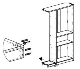
10, a. The 22 and 23 are connected to the 1 with (10). b. The 19 is connected with the 1 by (1), (2) and (10). Note: The cabinet can be put down to fix the buckle wheel under the 3.
