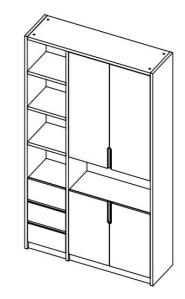
, fastener holes pasted (16), insert the drawer, adjust the distance between the drawer and the door panel to 2mm, the installation is complete
