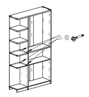
11. Insert the 25, then connect the 26,24 to the 1with (1) and (2).
