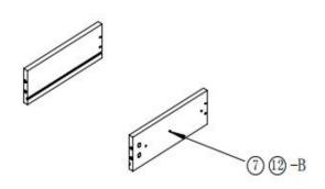
6、 Use ⑦ to install sliding rail ⑫-B on the outside of the 11 and 12.
