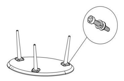
Use screw, flat washer, spring washer (as shown in the picture) to install the leg on the table top, the installation is complete
