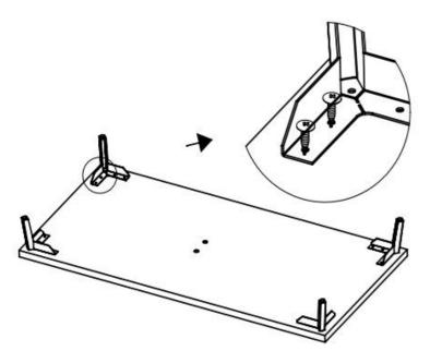
1. Metal leg (17) are installed under the 9 with (7).
