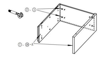
7、 a. Install rail (18)-A on the inside of the 1 and 6 with (7). b. The 16 is connected and fixed respectively with the 1 and 6 using the (2) and (1).
