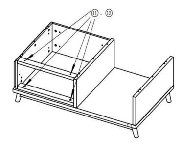
9, The 9 use (1) and (2) are installed on the 3 and 4.
