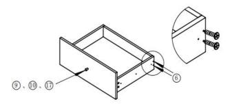
13、 Use (6) to connect and fix the10,11 and 12.(9) and (10) are used to connect the (17) on the 2.
