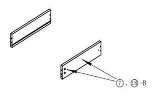
11、 Install rail 18-B on the outside of the 10 and 11 by using ⑦.
